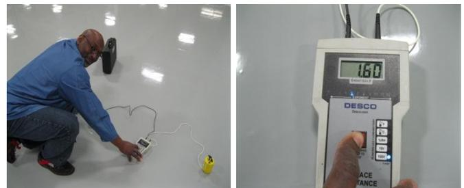
*Floropoxy ESD being tested with megohmmeter.*
